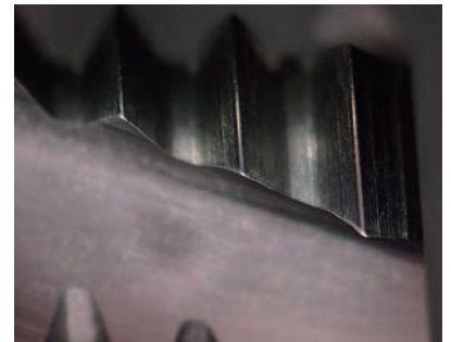
No.2 (after cutting 8,800 threads)
