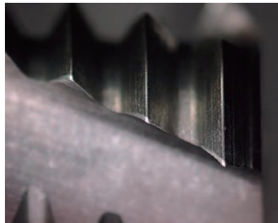
No.1 (after cutting 8,800 threads)
