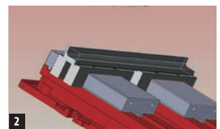
1. CAD / CAM model of a part made from 13-8 stainless steel. Image courtesy of Allied Tool & Die.
